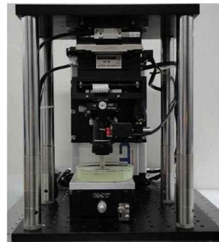
Fig. 3 MSTL using blu-ray optical pickup unit
