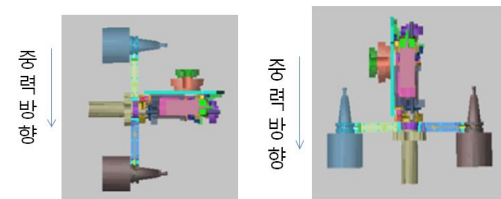
Fig. 2 Horizontal & Vertical Alignment
