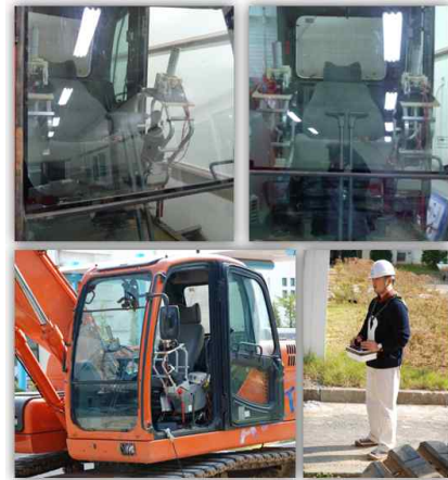
Fig. 3 Installed remote control system
