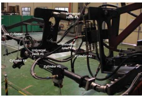
Fig. 5 Neck mechanism
