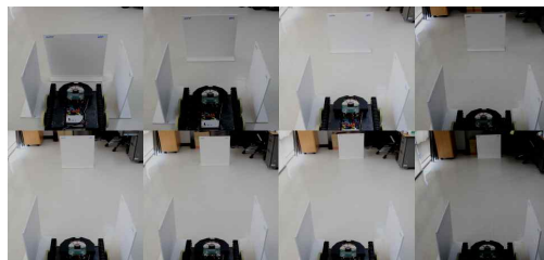
Fig.3 Sensing test of different obstacle distances
