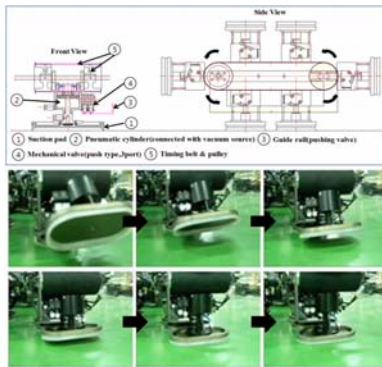
Fig. 3 Tracked wheel mechanism
