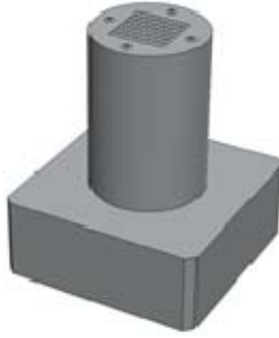
Fig.2 Solid model of fly eye lens mold core
