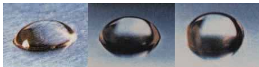
Fig. 6 Water Repellent Test
