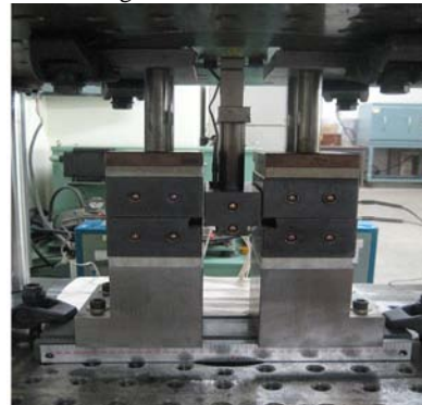
Fig. 1 The equipment of U-bending punch and die
