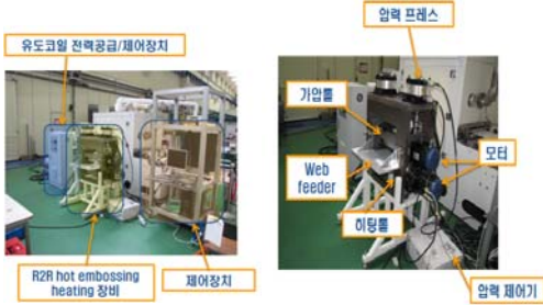
Fig. 3 Hot embossing R2R system.
