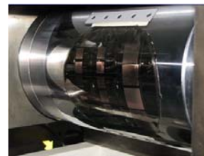
Fig. 2 Fabricated Ni stamp fastened on the roll.
