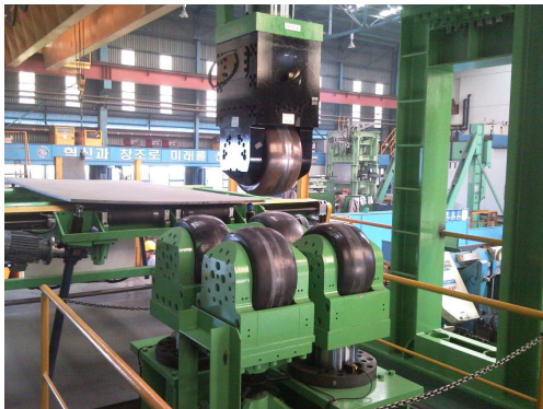
Fig. 2 Developed roll forming system
