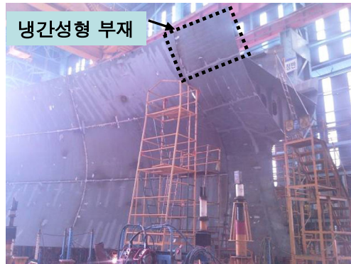
Fig. 3 Block assembly of formed plate
