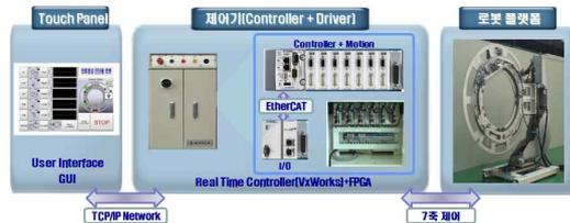
Fig. 3 Motion Controller for Imbalanced Rotor for a Medical Imaging Robot
