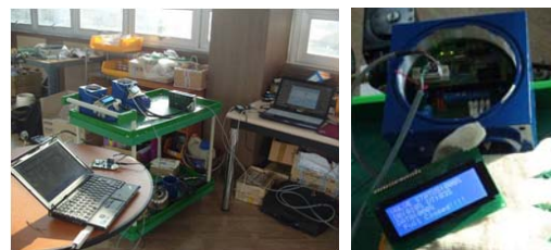
Fig. 5 Power line communication test using PLDSK
