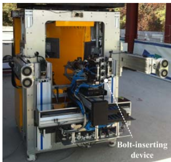
Fig. 1 Bolting robot system with bolt-inserting device
