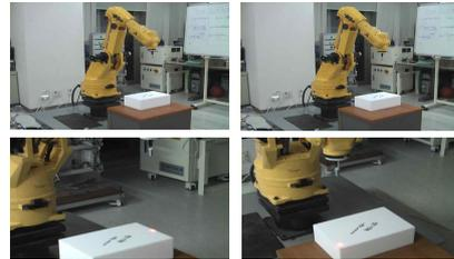
Fig. 4 The manipulator operates the task for tracking the edges of a rectangular parallelepiped.
