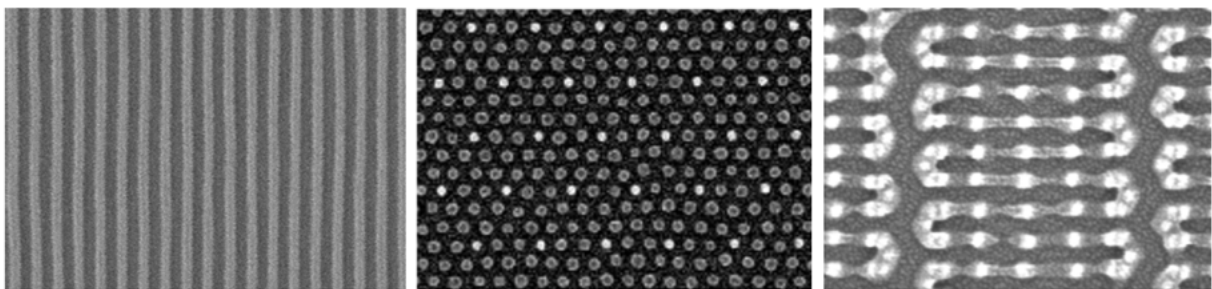
Figure 1. Various kinds of silica nanopatterns prepared with Si-containing block copolymers.
