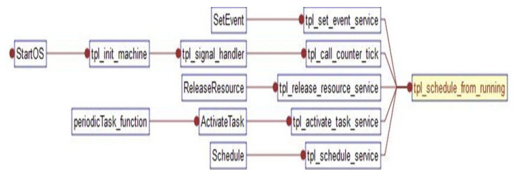
(Figure 2) Demonstrating Root Function Reference for tpl_schedule_from_running , using Understand API
