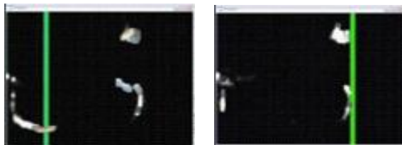
Fig 3. Shows the scan line that is moving from left to right. Any non-zero pixel that it meets will play a note assigned to that location.
