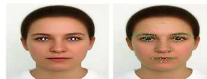
Fig.2. Input image & both eyeballs used for normalization(left) normalized image & pre-defined 61 facial features(right)
