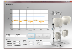
Fig.5 GUIO program for Torque test equipment
