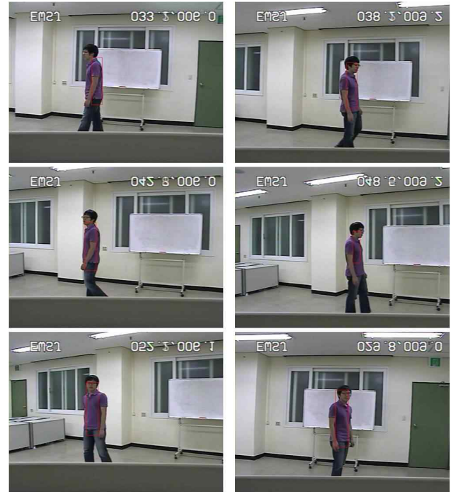
Fig. 3 Tracking results. The moving object is located at the center in the camera image, since the camera tracks the moving object.
