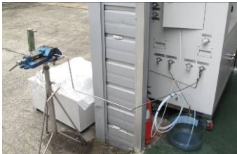
Fig. 8 Configuration of Cooling Channel Specimen with Attached Strain Gauge
