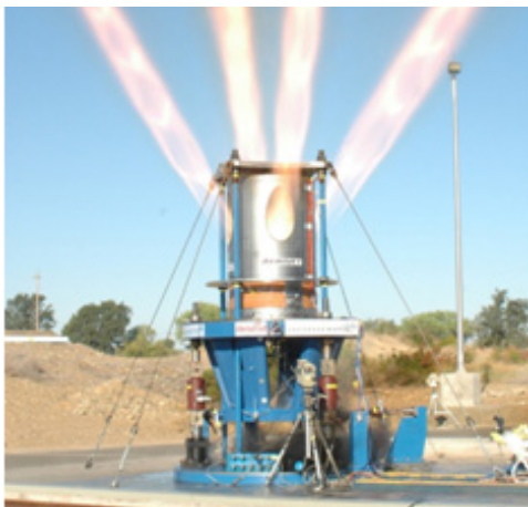
Fig. 3 Ullage motor of Saturn-V
