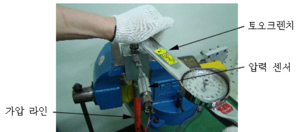
(b) Nozzle closure assembling
