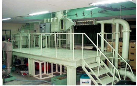
Fig. 2 CNU high speed cavitation tunnel
