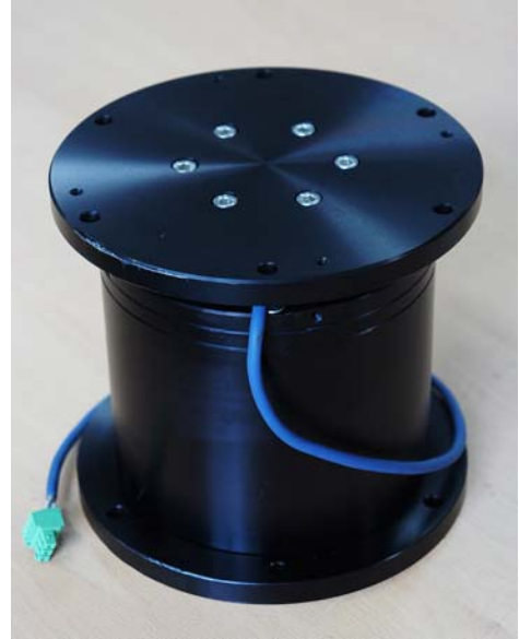
Fig. 6 Photograph of the manufactured MR damper
