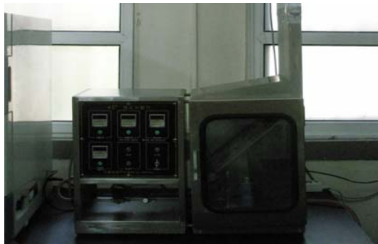
Figure 1. A photo of 45° combustion tester
