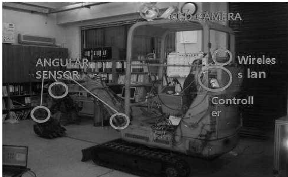
Fig. 1 Appearance of Tele-operated Excavator
