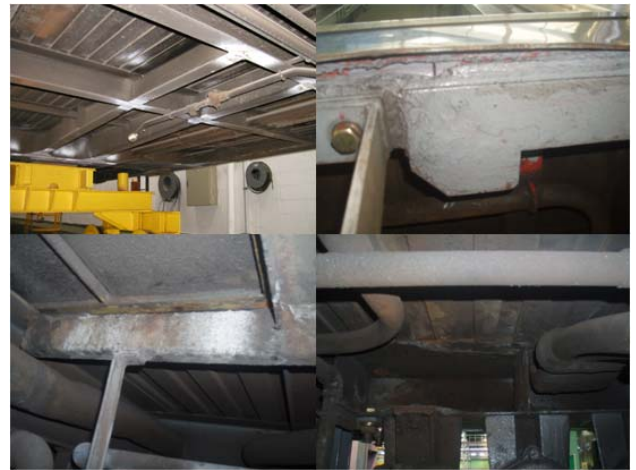
Fig. 1 Corrosion of car-body structure
