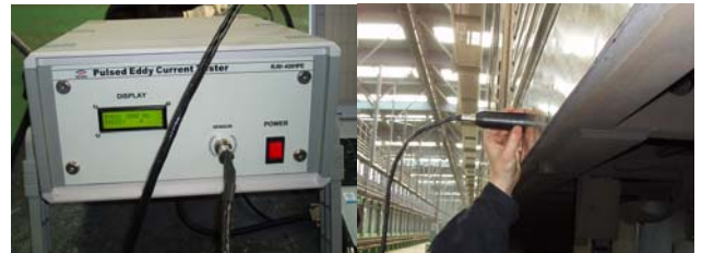
Fig. 5 Pulse - eddy current testing
