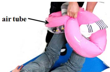
Fig. 3 A simplified test of air tube concept for ankle clamp
