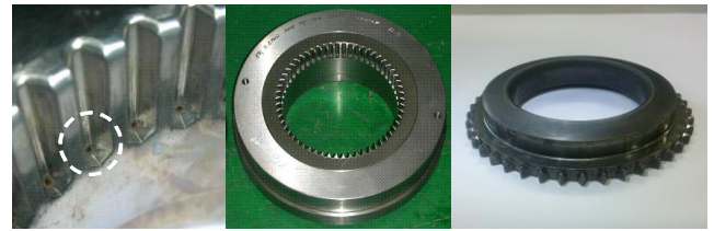
(a) Die with air-hole (b) Clutch gear part Fig. 8 Experiment result
