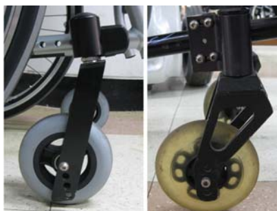
Fig6. Angle of the Caster Fork
