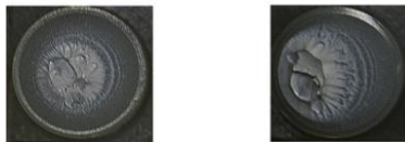
(a) Symmetric crack (b) Asymmetric crack
