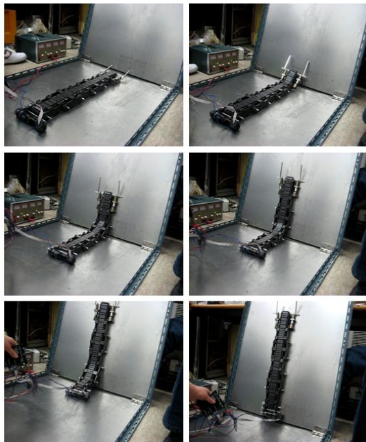
Fig. 4 Wall-to-wall transition driving (angle between wall surfaces: 80° )
