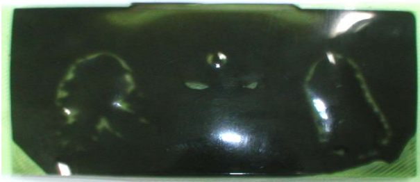
Fig. 3 Surface of microcellular injection molding product using PP Polymer film
