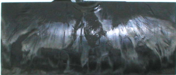
Fig. 4 Surface of microcellular injection molding product using Tefron Polymer film
