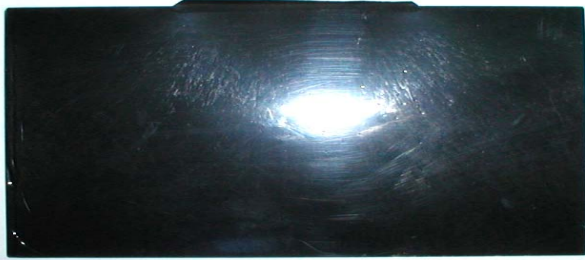
Fig. 2 Surface of microcellular injection molding product using APET Polymer film
