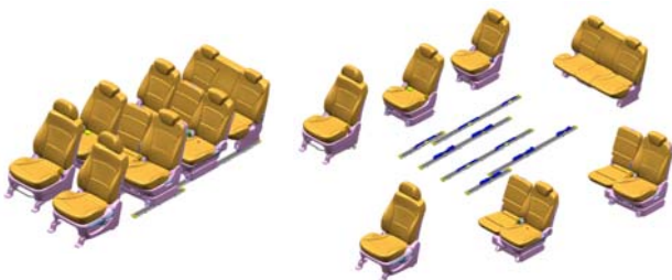
(a) Seat Lay-out (b) Arrangement of Sliding Seat
