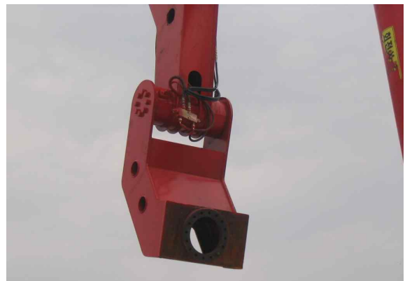
Fig. 8 Application of rolling type hydraulic cylinder
