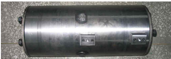
Fig. 5 Prototype of rolling type hydraulic cylinder
