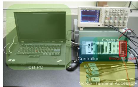
Fig. 2 Structure of Pitch Bearing Deformation Monitoring System
