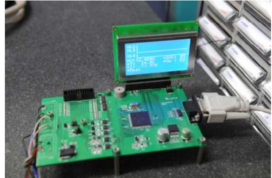
Fig 2. Bosch battery sensor interface board
