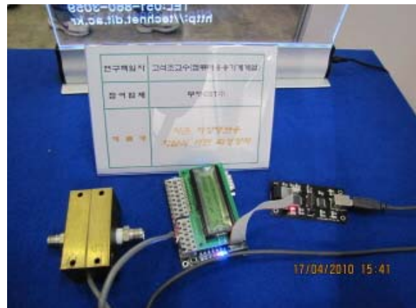
Fig. 4 Picture of implemented digital level meter
