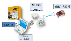
Fig 2. construction of System
