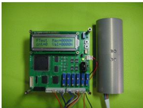
Fig. 4 Manufactured cylindrical object measuring system
