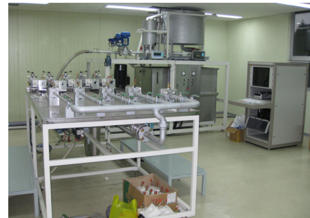
Fig.1 Calibration system for water meters
