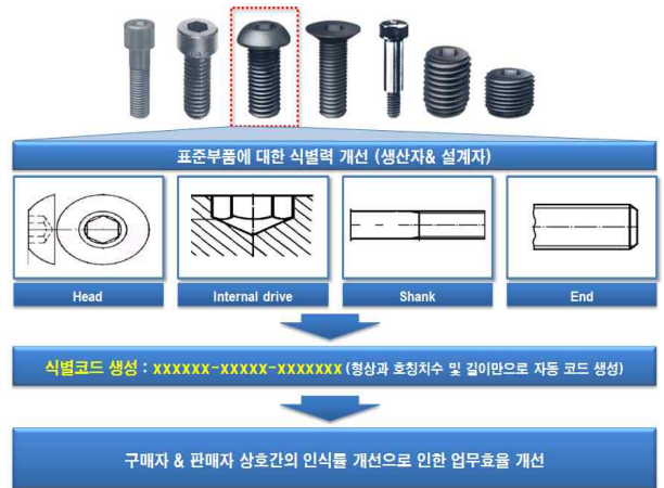
Fig. 2 Identification grant method of bolt through shape
