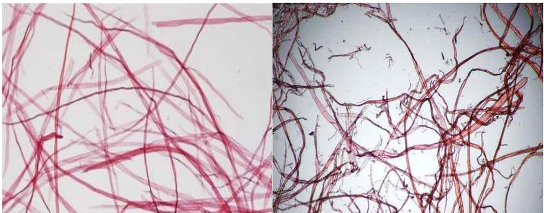
Fig. 2. UKP before kneading pretreatment( $\times 40$ ). Fig. 3. UKP after kneading pretreatment( $\times 40$ ).
