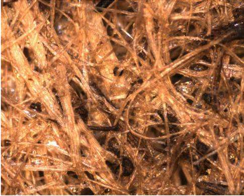
**Fig. 4. Surface structure of cushioning materials made of palm fibers.**
