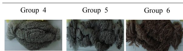
Fig. 2. Comparison of 3-combination dye adsorption compatibility on PLA with conventional disperse dye sets using PET, acetate dyeing.
