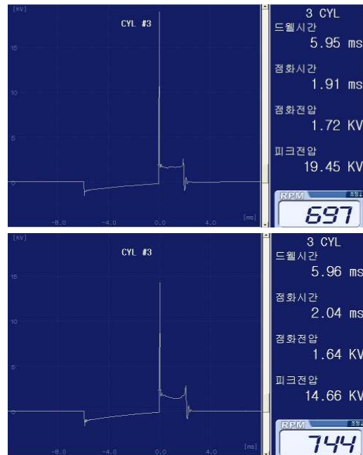
Fig. 9 Spark-plug gap (Top: abnormal, Bottom: normal)
