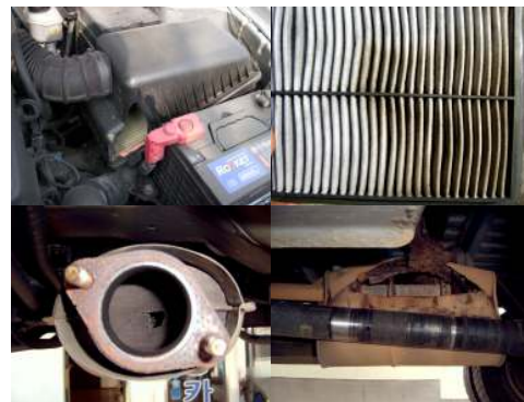
Fig. 3 Damages by engine backfire
