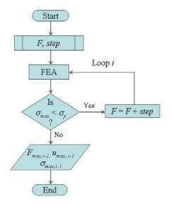
Fig. 4. Procedure for the FEA simulation of the crab pot frame.
