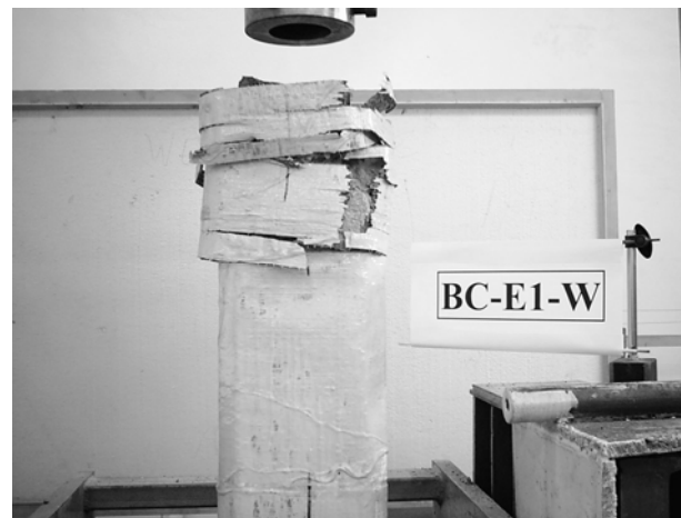
Fig. 5. Failure of confined concrete column.
